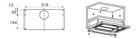
**Step 1:** The rangehood should be placed at a minimum distance of 65cm above the cooking surface when placed above an electric hob and a minimum of 75cm above the cooking surface when placed above a gas cooktop.
